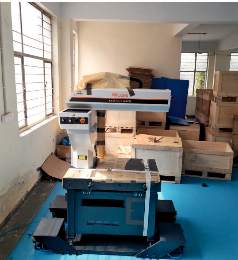
MITUTOYO MISTAR CMM INSTALLED ON DYNEMECH MEMBRANE AIR SPRING WITH INERTIA MASS IN LNM AUTO-FARIDABAD
