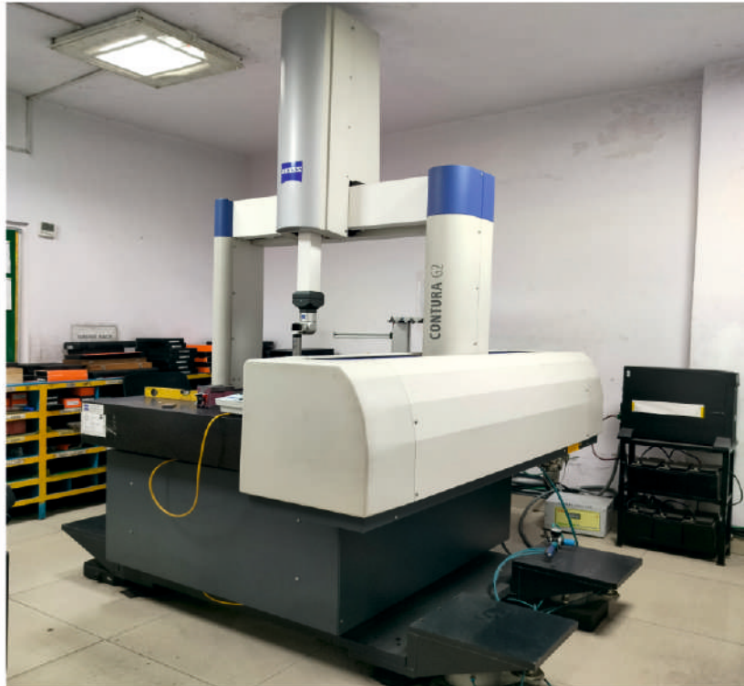
CARL ZEISS CONTURA G2 INSTALLED ON DYNEMECH MEMBRANE AIR SPRING WITH INERTIA MASS IN BLUE STAMPING-FARIDABAD
