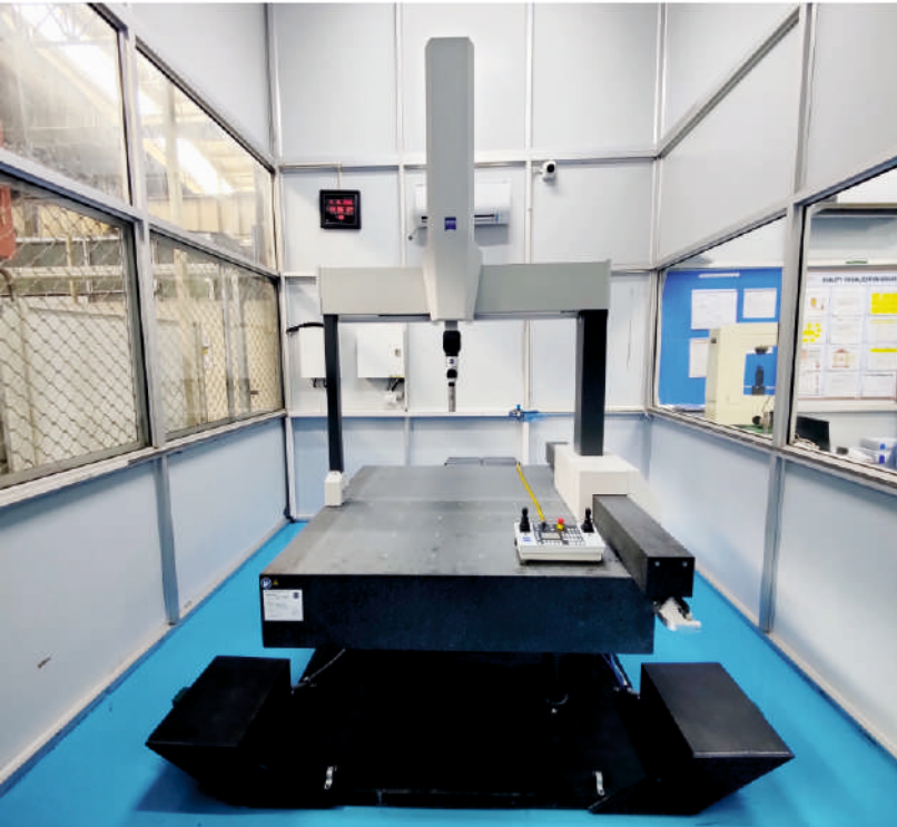
CARL ZEISS SPECTRUM 10-12-8 INSTALLED ON DYNEMECH MEMBRANE AIR SPRING WITH INERTIA MASS IN PPAP AUTOMOTIVE-GREATER NOIDA
