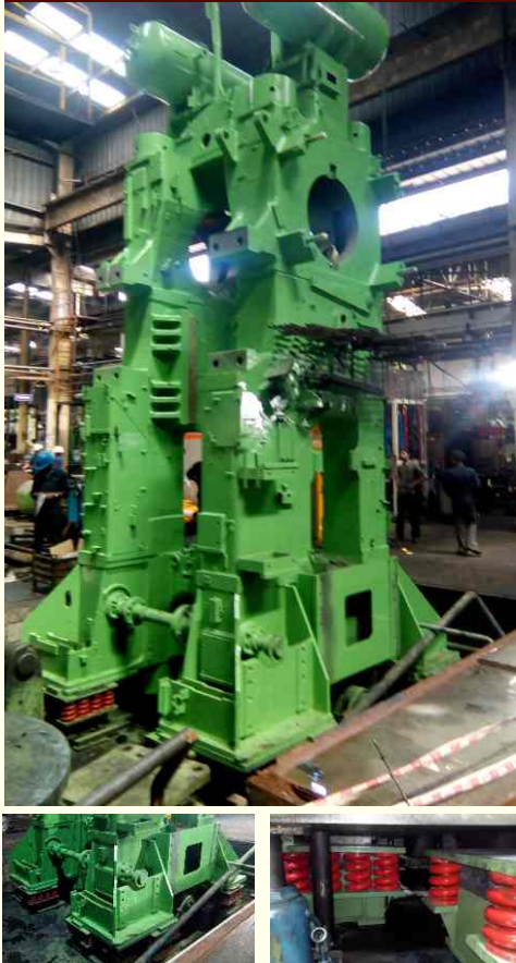
FORGING PRESS MOUNTED ON SPRING ISOLATORS
