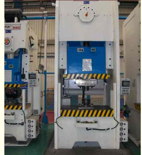
POWER PRESS ON SPRING ISOLATORS
