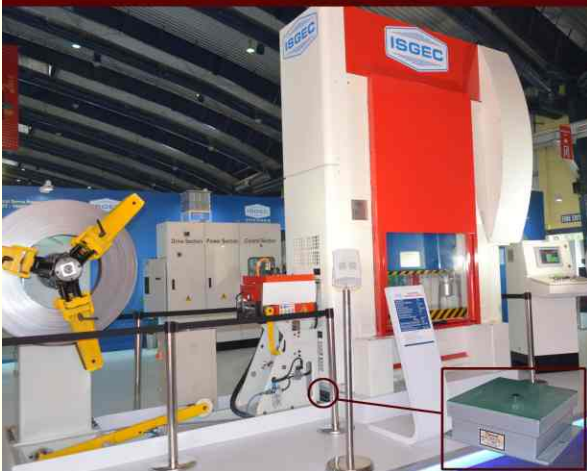
63 TON HIGH SPEED PRESS ON DYNEMECH SPRING ISOLATORS
