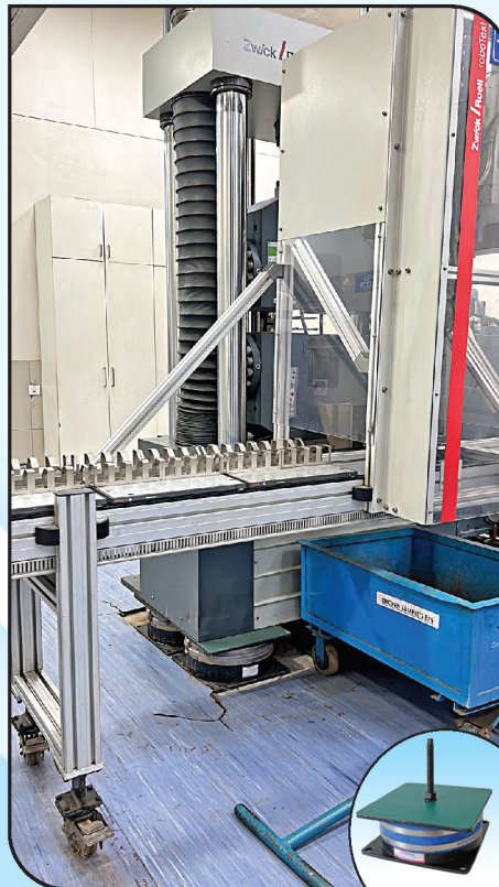
Zwick 100 ton Universal Test Machine on Spring Viscous Dampers protected from External Vibrations
