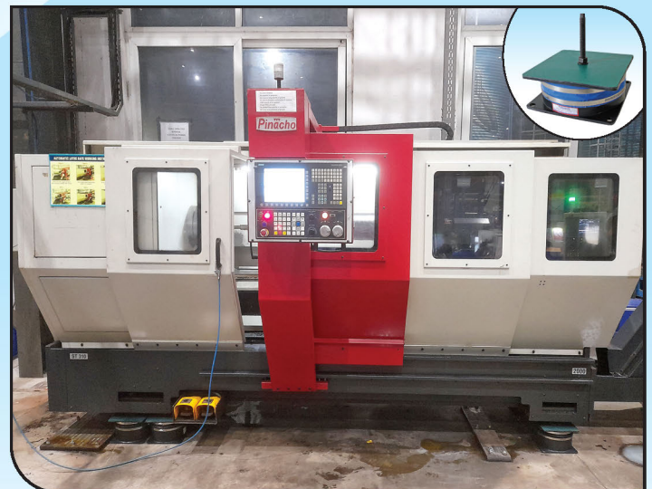
CNC Lathe installed on suspended slab using Spring Viscous Dampers
