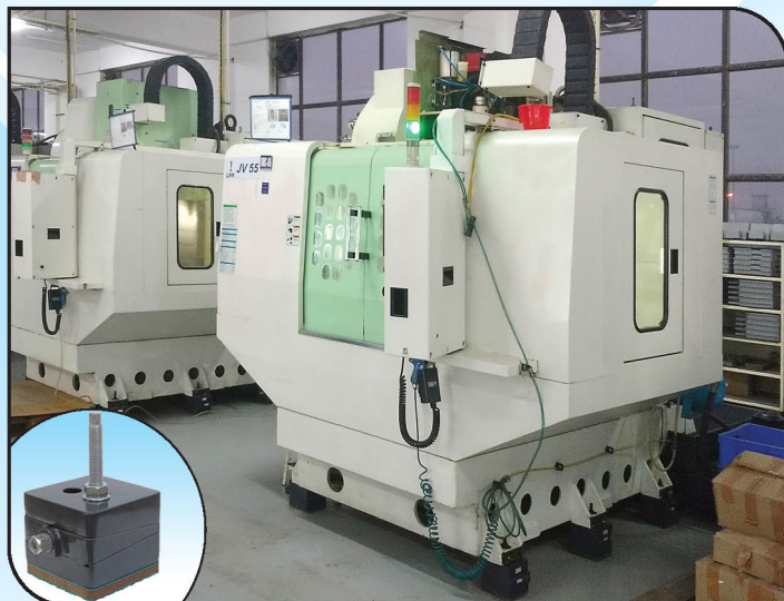
VMC Machine installed on suspended slab on Dynemech Wedge Mount Series DBP
