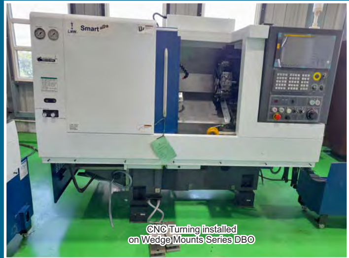
CNC Machine Center installed on Wedge Mounts Series DBO
