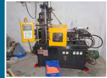
Injection Molding Machine installed on DLK
