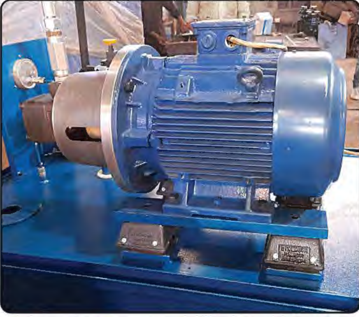
Motor on Dynemech Flexifoot Mounts
