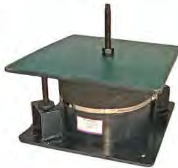
2250KVA GENSET 15500Kg on Restrained Spring Isolator with Safety Viscous Damping
